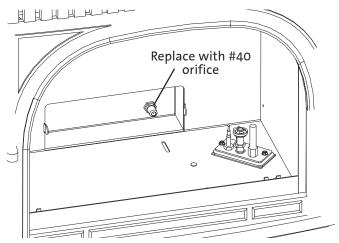
Figure 43. Change the Burner Orifice.
